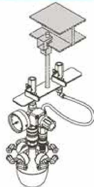
■Bolts and hanging fixture are not included and need to be prepared by customers. ■The diameter of hole on the plate is 11 mm. ■Rc 1/4" threaded connection.
