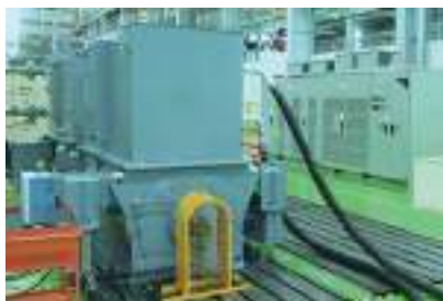
Combined test with inverter drive
