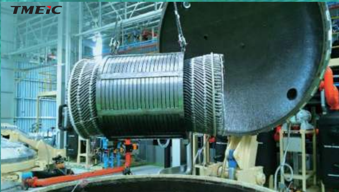
Installing stator in VPI tank
